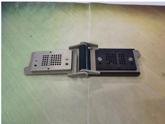
Illustration 10: Punch die for repairing punched tape © ISL
